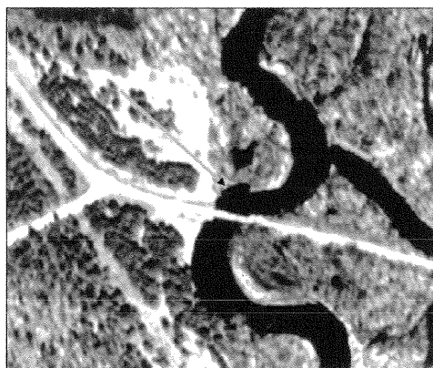
Figure 4: Infrared air photograph from 2000 showing bank scour (at green arrow) due to the narrow span of the bridge constructed c. 1917.
